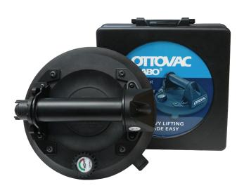
OTTOVAC is a portable electric vacuum lifting device intended to lift and move material that has a smooth, flat and non-porous surface. The OTTOVAC has a built-in pressure sensor with an automatic start/stop function. When the vacuum in the base of the suction cup reaches - 55 kPa, the pump will automatically stop after a three-second delay. When the vacuum level drops below -55 kPa, the pump will automatically restart, reaching the required pressure during operation.
